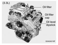
The engine oil and filter should be changed at those intervals specified in the maintenance schedule in Section 5. If the car is being driven in severe conditions, more frequent oil and filter changes are required.
