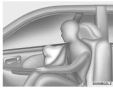
Your Hyundai is equipped with a side impact airbag in each front seat. The purpose of the airbag is to provide the vehicle's driver and/or the front passenger with additional protection than that offered by the seat belt alone. The side impact airbags are designed to deploy only during certain side-impact collisions, depending on the crash severity, angle, speed and point of impact. The side impact airbags are not designed to deploy in all side impact situations.
