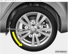
The wheel nuts should be loosened slightly before raising the car. To loosen the nuts, turn the wrench handle counterclockwise. When doing this, be sure that the socket is seated completely over the nut so it cannot slip off. For maximum leverage, position the wrench so the handle is to the left as shown in the drawing. Then, while holding the wrench near the end of the handle, push down on it with steady pressure. Do not remove the nuts at this time. Just loosen them about one-half turn.
