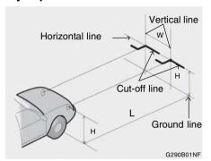
If the vehicle has had front body repair and the headlight assembly has been replaced, the headlight aiming should be checked using the aiming screen as shown in the illustration. Turn on the headlight switch (Low Beam Position).
