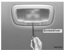
Remove the plastic cover with a flathead screwdriver.
