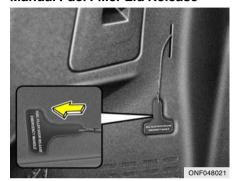
If the fuel filler lid cannot be opened using the remote opener, a manual opener handle is located inside the trunk on the left side. Open the fuel filler lid by pulling on this handle as shown in the illustration.
