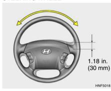
To check the steering wheel free-play, stop the car with the wheels pointed straight ahead and gently move the steering wheel back and forth. Use very light finger pressure and be sensitive to changes in resistance that mark the limits of the free-play. If the free-play is greater than specified, have it inspected by your Hyundai dealer and adjusted or repaired if necessary.
