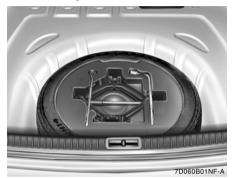
Take out the tool receptacle and turn the installation bolt counterclockwise to remove spare tire from the trunk.
