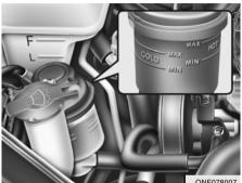
The power steering fluid level should be checked regularly. To check the power steering fluid level, be sure the engine is "OFF", then check to make certain that the power steering fluid level is between the "MAX" and "MIN" level markings on the fluid reservoir.
