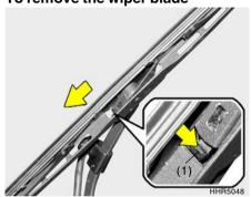
Push down the wiper blade with the locking clip (1) pressed to detach it from the wiper arm.
