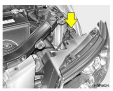
5. Disconnect the power cord from the back of the headlight.
