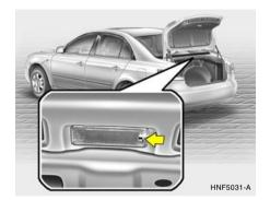
2. Remove the luggage compartment light cover on the rear package tray panel with a flat-head screwdriver.
