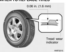
The original tires on your car have tread wear indicators. The location of tread wear indicators is shown by the "TWI" or "\(\triangle \)" marks, etc. The tread wear indicators appear when the tread depth is 0.06 in. (1.6 mm). The tire should be replaced when these appear as a solid bar across two or more grooves of the tread. Always replace your tires with those of the recommended size. If you change wheels, the new wheel's rim width and offset must meet Hyundai specification.
