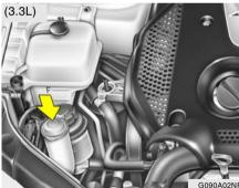
The washer fluid reservoir supplies fluid to the windshield washer system.
