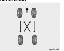
Tires should be rotated every 7,500 miles (12,000 km). If you notice that tires are wearing unevenly between rotations, have the car checked by a Hyundai dealer so the cause may be corrected.
