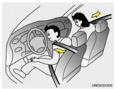
Your Hyundai vehicle is equipped with driver's and front passenger's pre-tensioner seat belts. The purpose of the pre-tensioner is to make sure that the seat belts fit tightly against the occupant's body in certain frontal collisions. The pre-tensioner seat belts can be activated alone or, where the frontal collision is severe enough, together with the airbags.
