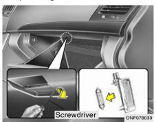
2. Remove the glove box illuminated light cover with a flat-head screwdriver.
