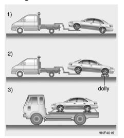
Your vehicle can be towed by wheel lift type truck (1), (2) or flatbed equipment (3).
