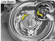
Remove the protective cap from the replacement bulb and install the new bulb by matching the plastic base with the headlight hole.
