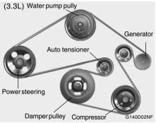
Drive belts should be checked periodically for proper tension. At the same time, belts should be examined for cracks, wear, fraying or other evidence of deterioration and replaced if necessary.
