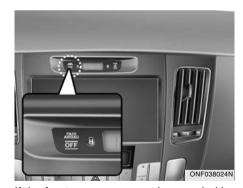
If the front passenger seat is occupied by a person that the system determines to be of adult size, and he/she sits properly (sitting upright with the seatback in an upright position, centered on the seat cushion with their seat belt on, legs comfortably extended and their feet on the floor), the "PASSENGER AIR BAG OFF" indicator will be turned off and the front passenger's air bag will be able to inflate, if necessary, in frontal crashes.
