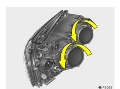
6. Turn the plastic cover counterclockwise and remove it.
