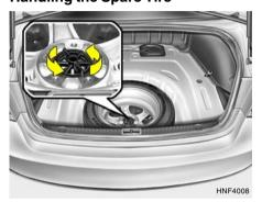
To remove the spare tire, take out the tool receptacle and remove the installation bolt by turning it counterclockwise. After replacing the spare tire, install and tighten the bolt firmly with your fingers until there is no more play in the spare tire.
