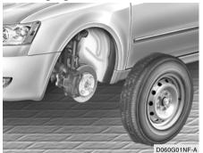
Loosen the wheel nuts and remove them with your fingers. Slide the wheel off the studs and lay it flat so it cannot roll away. To put the wheel on the hub, pick up the spare tire, line up the holes with the studs and slide the wheel onto them. If this is difficult, tip the wheel slightly and get the top hole in the wheel lined up with the top stud. Then jiggle the wheel back and forth until the wheel can be slid over the other studs.
