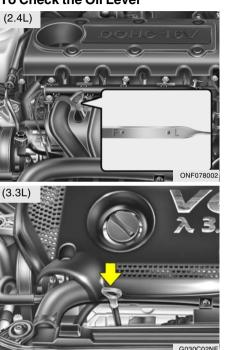
Before checking the oil, warm up the engine to the normal operating temperature and be sure your car is parked on level ground. Turn the engine off.
