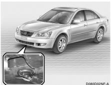
For emergency towing when no commercial tow vehicle is available, attach a tow cable, chain or strap to the towing hook under the front of your car. Do not attempt to tow your vehicle in this manner on any unpaved surface. This could result in serious damage to your car.
