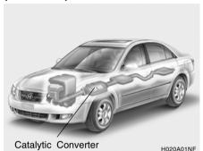
Hyundai vehicle is equipped with a monolith type three-way catalytic converter to reduce the carbon monoxide, hydrocarbons and nitrogen oxides contained in the exhaust gas. Exhaust gases passing through the catalytic converter cause it to operate at a very high temperature. The introduction of large amounts of unburned gasoline into the exhaust may cause the catalytic converter to overheat and create a fire hazard. This risk may be reduced by observing the following:
