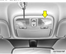
1. Remove the plastic cover with a flathead screwdriver.
