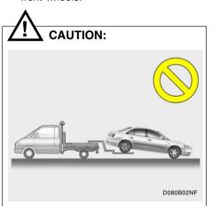
A vehicle with an automatic transaxle should never be towed from the rear with the front wheels on the ground. This can cause serious damage to the transaxle.
