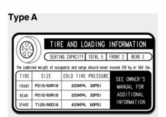
These pressures were chosen to provide the most satisfactory combination of ride comfort, tire wear and stability under normal conditions. Tire pressures should be checked at least monthly. Proper tire inflation pressures should be maintained for these reasons:
