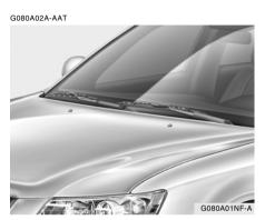
The wiper blades should be carefully inspected from time to time and cleaned to remove accumulations of road film or other debris. To clean the wiper blades and arms, use a clean sponge or cloth with a mild soap or detergent and water. If the wipers continue to streak or smear the glass, replace them with genuine Hyundai replacement parts or their equivalent.
