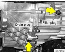
Transaxle lubricant in the manual transaxle should be checked at those intervals specified in the vehicle maintenance schedule in Section 5.
