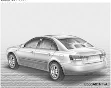
In addition to the lower-mounted rear stop lights on either side of the car, the high mounted rear stop light in the center of the rear window also lights when the brakes are applied.
