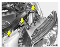
Using a socket wrench of the correct size, remove the headlight assembly mounting bolts and bumper mounting bolt.
