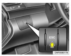
The Electronic Stability Control (ESC) system is designed to stabilize the vehicle during cornering manuevers. ESC checks where you are steering and where the vehicle is actually going. ESC applies the brakes at individual wheels and intervenes in the engine management system to stabilize the vehicle.
