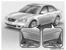
The base of the jack should be placed on firm, level ground. The jack should be positioned as shown in the drawing. D060F02E-AAT
