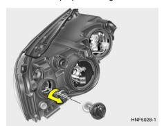
12. To replace the front turn signal light bulb remove it from the bulb holder and install the new bulb.
