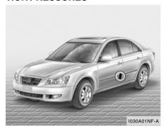
Tire label located on the driver's side center pillar outer panel gives the cold tire pressures recommended for your vehicle with the original tire size, the number of people that can be in your vehicle and vehicle capacity weight.
