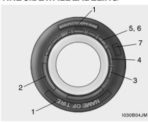
Federal law requires tire manufacturers to place standardized information on the sidewall of all tires. This information identifies and describes the fundamental characteristics of the tire and also provides the tire identification number (TIN) for safety standard certification. The TIN can be used to identify the tire in case of a recall.
