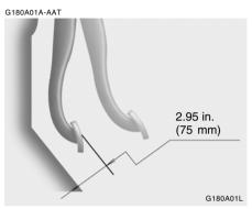
You need a helper to check the brake pedal clearance. With the engine running, have your helper press down on the brake pedal several times and then hold it down with a force of about 110 lbs (50 kg, 490 N). The brake pedal clearance is the distance from the top surface of the brake pedal to the asphalt sheeting under the floor mat. If the brake pedal clearance is not within the limits specified in the illustration, have it inspected by your Hyundai dealer and adjusted or repaired if necessary.
