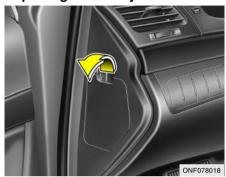
The fuse box for the lights and other electrical accessories will be found on the left side of the instrument panel. Inside the box you will find a list showing the circuits protected by each fuse.
